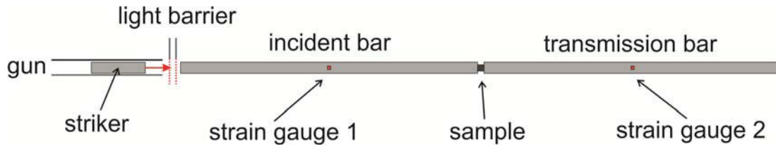
Fig. 1: Principal setup of the SHPB facility.
