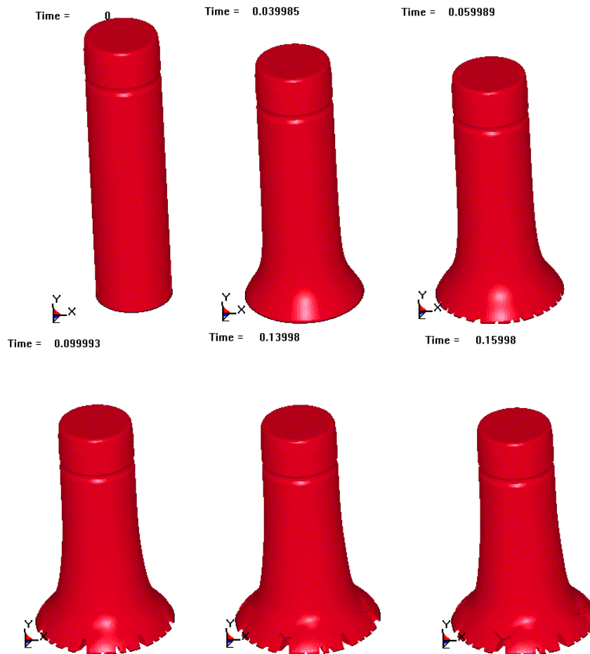
Fig. 15: Deformation failure process of 45 steel Taylor impact specimen (310m/s).
