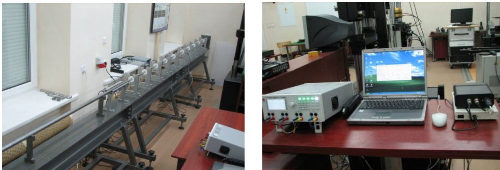
Fig. 3: Split Hopkinson Pressure Bar apparatus with data acquisition and control systems.
