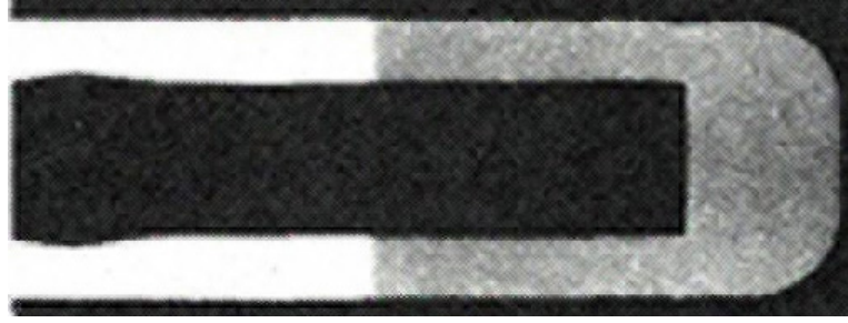
Figure 7: Flash X-radiograph taken 20 \mu s after symmetric Taylor impact at 127 m/s of 9mm diameter 35mm long tungsten alloy rods. From [23].
