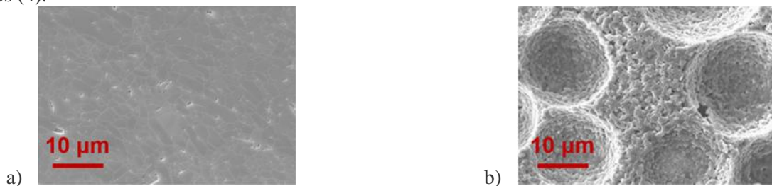
Figure 1: Characteristic SEM observations of two grades of the studied alumina ceramics –a) A-Grade (porosity ratio near 0%) and b) B-Grade (porosity ratio of about 60%)
