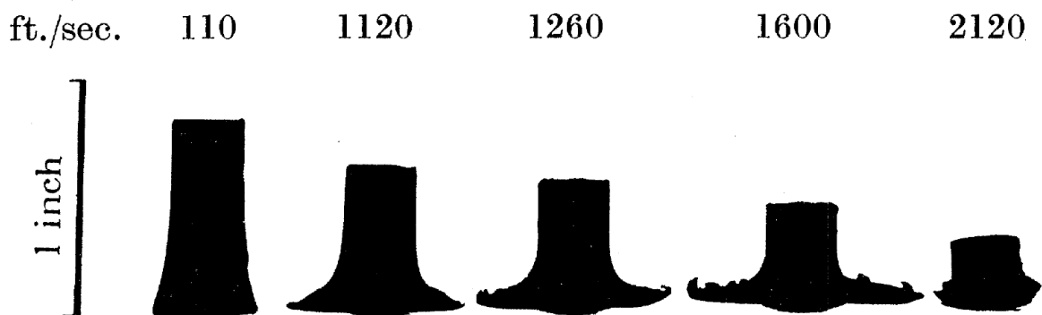
Figure 1: Shadowgraph images of cylindrical mild steel specimens (originally 1 inch long and 0.3 inches diameter) after impact on 'heavy armour' plates at various speeds. From [1].
